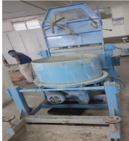
Fig. 1. Pan mixer Used for concrete Blending.
