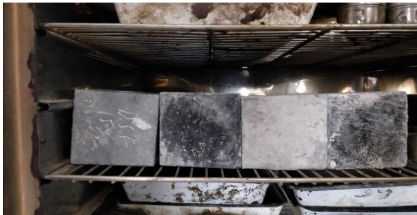
Fig. 27. Cubes placed in oven for desorption test.
