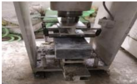
Fig. 19. Flexural Strength test.
