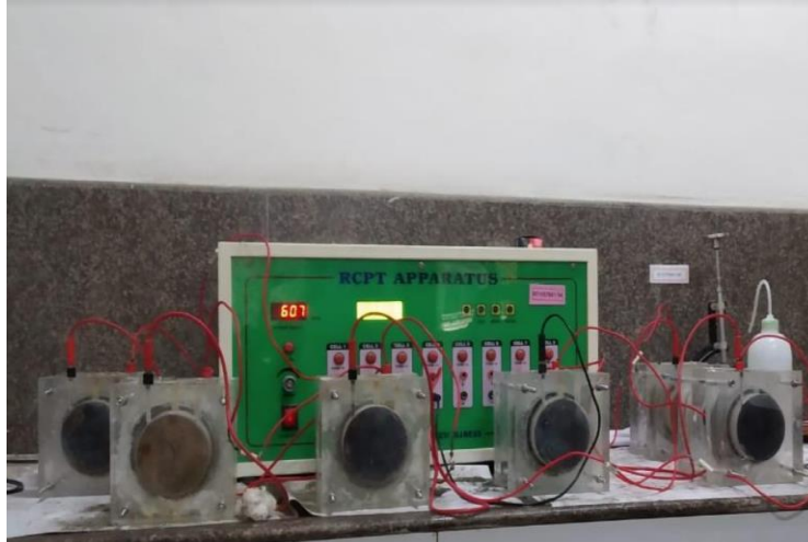
Fig. 5. RCPT test setup.
