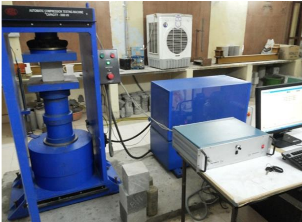
Fig. 16. Compressive strength test.
