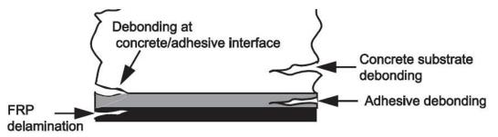
Fig. 1. Different interface crack initiation possible phases [26].
