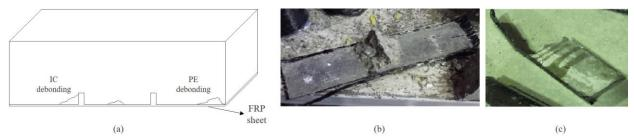
Fig. 5. a) Modes of debonding b) IC debonding, and c) PE debonding.
