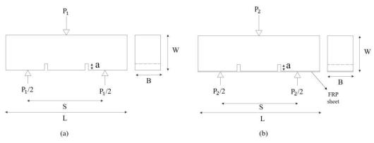
Fig. 6. a) Un-retrofitted specimen, b) Retrofitted specimen
