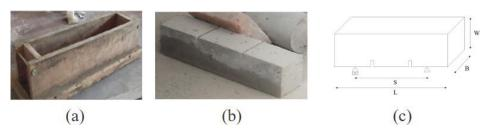
Fig. 2. Specimen a) mold, b) notched form, and c) dimensions.
