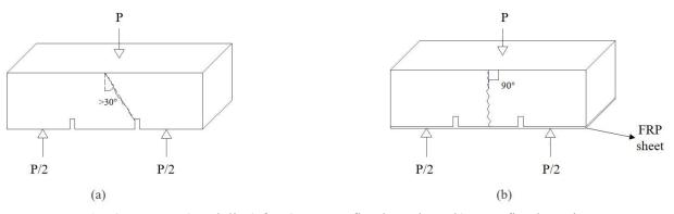
Fig. 4. Fracture (crack line) for a) un-retrofitted specimen b) Retrofitted specimen.
