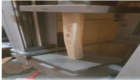
Fig. 4. The failure mode of Iroko (600mm).
