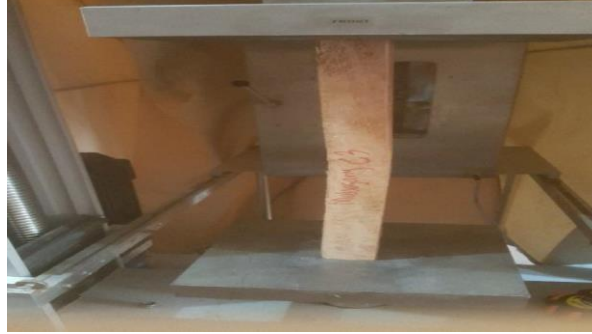
Fig. 3. The failure mode Mahogany (600mm).
