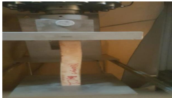
Fig. 2. Failure mode Mahogany (400mm).
