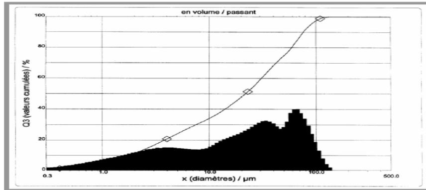
**Fig. 2.** Particle size distribution of the slag.
