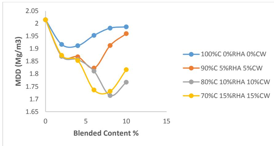
**Fig. 6.** Relationship between the MDD of laterite treated with (100%C 0%RHA 0%CW), (90%C 5%RHA 5%CW), (80%C 10%RHA 10%CW) & (70%C 15%RHA 15%CW) blended cement.
