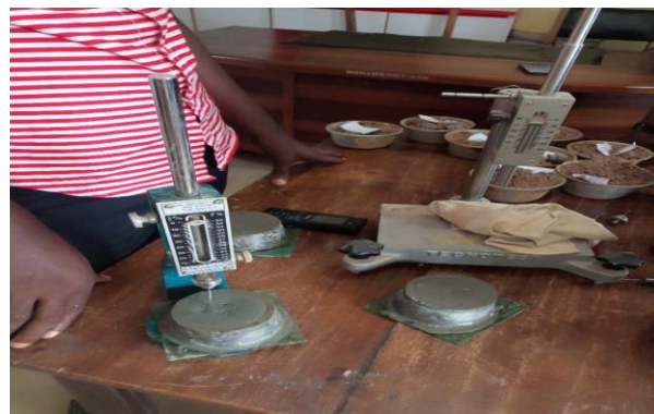
Fig. 2. Setting Time Laboratory Tests.
