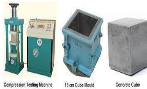
Fig. 1. Concrete cube for compressive strength testing.
