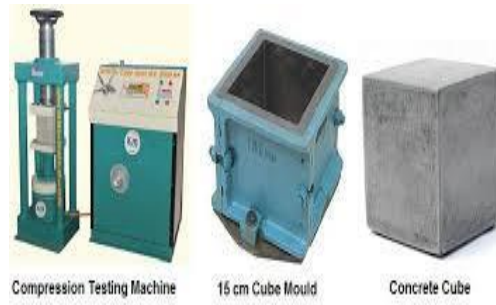
Fig. 1. Concrete cube for compressive strength testing.
