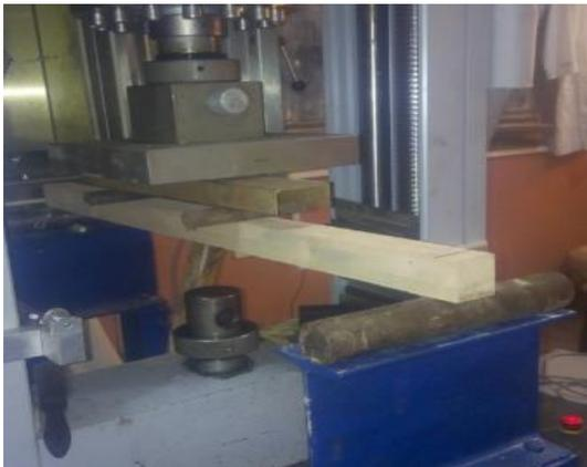
**Fig. 2.** 4-Point Bending test Setup.
