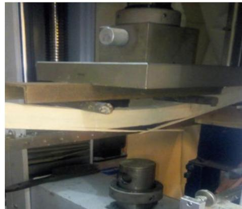
**Fig. 3.** Failure Mode of 4-point Bending Test.
