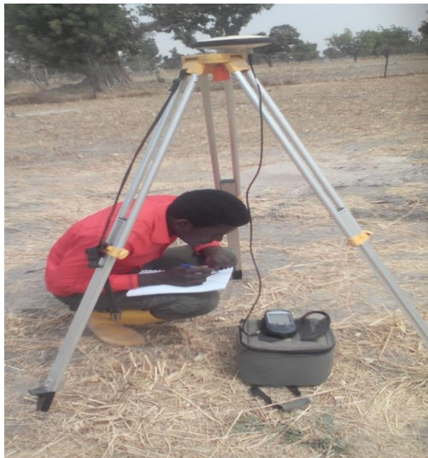
Fig. 2. Determining elevation in the research area using ProMark GPS System.
