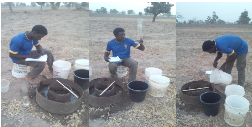
Fig. 4. Determining infiltration rate in the research area.
