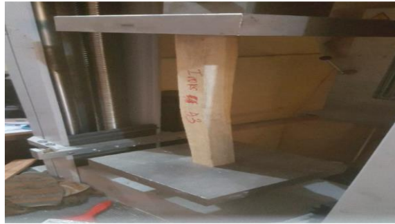
Fig. 4. The failure mode of Iroko (600mm).
