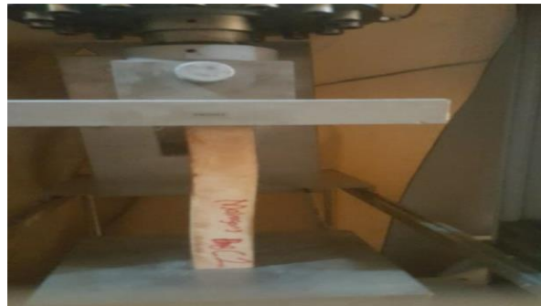
Fig. 2. Failure mode Mahogany (400mm).
