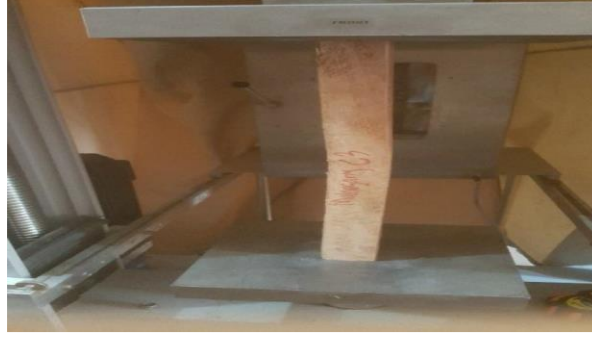
Fig. 3. The failure mode Mahogany (600mm).
