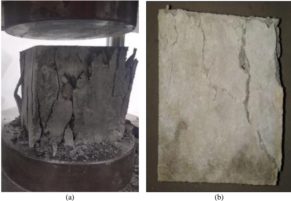
Fig. 6. Specimen after Compression failure (a) Plain Concrete (b) JRC4 (JF 0.1% & RH 10%).
