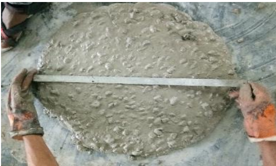
Fig. 1. Flow table test.
