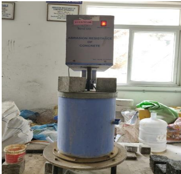
Fig. 10. Abrasion testing machine.
