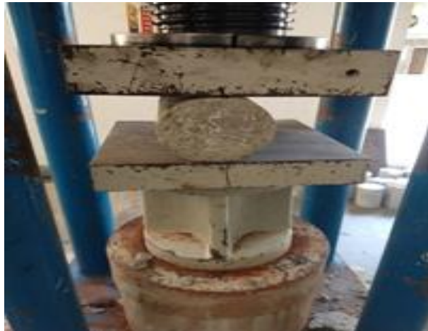
Fig. 9. split tensile strength testing machine.
