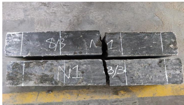
Fig. 7. Flexural strength test.
