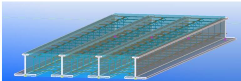
**Fig. 1.** Structure with concrete encased steel beams with I cross-section.
