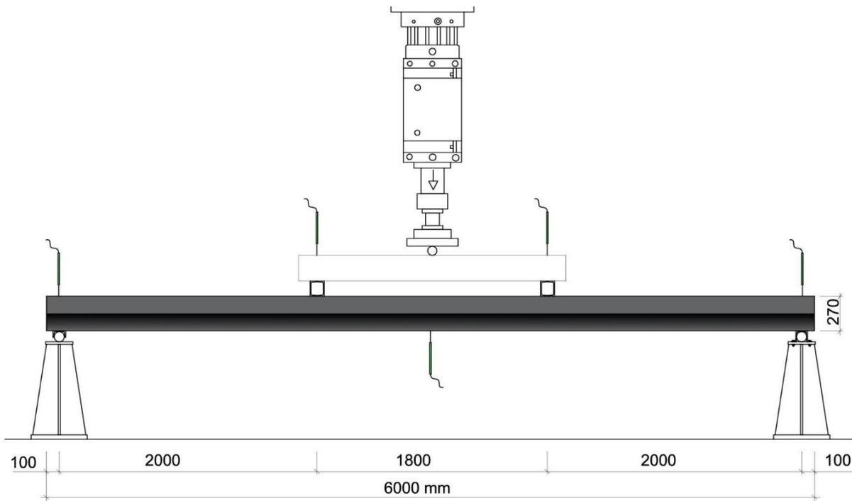
**Fig. 4.** Static scheme of composite beam and layout of sensors.
