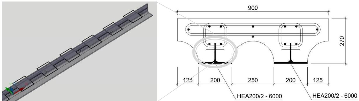
**Fig. 3.** Cross-section of beam NV2 with composite action using reinforcement loops.
