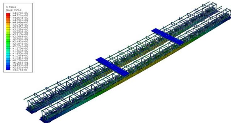
**Fig. 8.** Relative plastic behaviour of rigid steel reinforcement.
