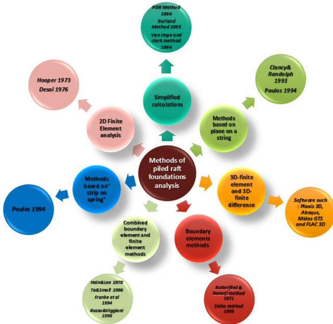
Fig. 2. Summary of the different methods of piled raft foundation analysis.
