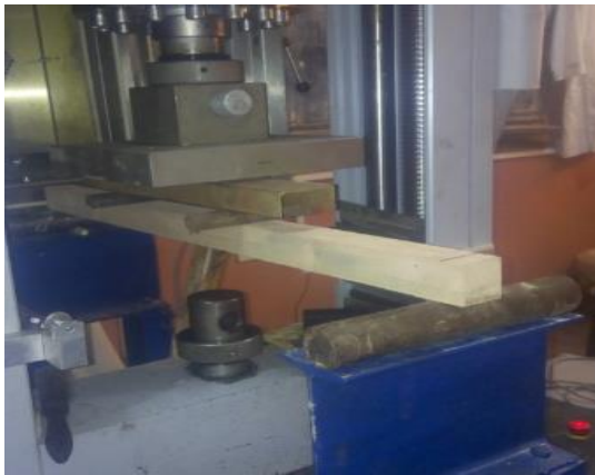
Fig. 2. 4-Point Bending test Setup.
