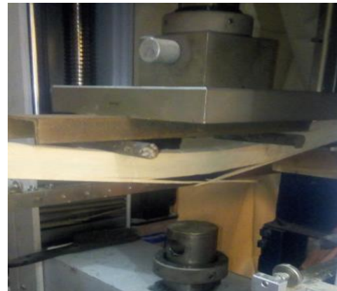
Fig. 3. Failure Mode of 4-point Bending Test.
